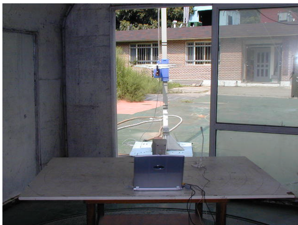
RADIATED EMISSION SETUP PHOTOGRAPH - REAR VIEW ( 300 - 1000 MHz )
