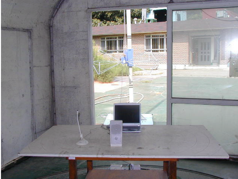
RADIATED EMISSION SETUP PHOTOGRAPH - FRONT VIEW ( 30 - 300 MHz )
