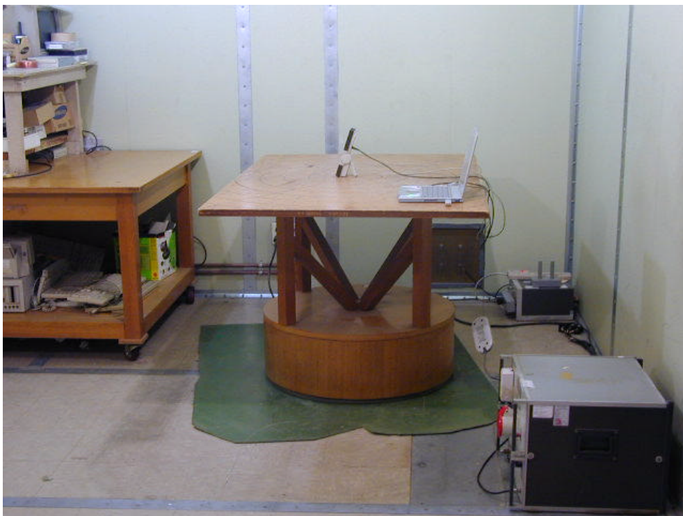
LINE CONDUCTED SETUP PHOTOGRAPH - REAR VIEW
