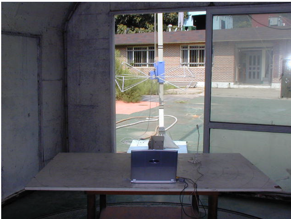
RADIATED EMISSION SETUP PHOTOGRAPH - REAR VIEW ( 30 - 300 MHz )
