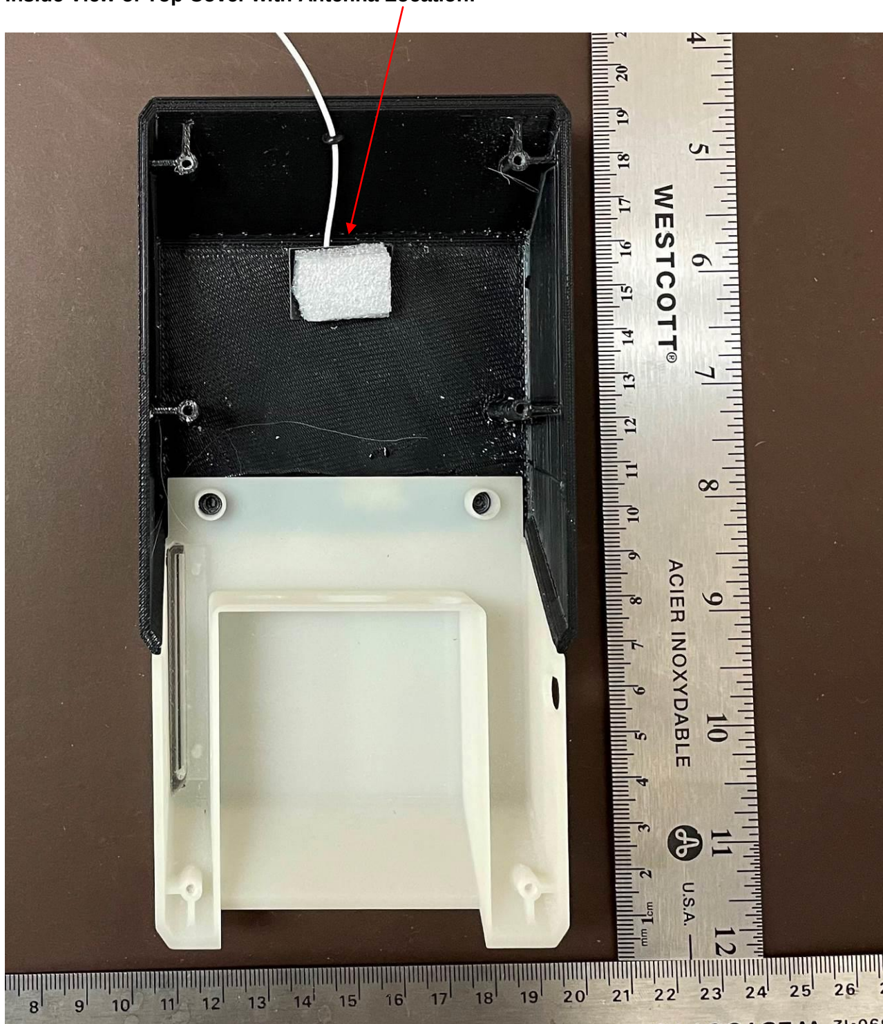
Inside View of Top Cover with Antenna Location:
