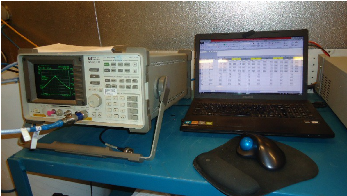
Figure 4.9 - Test Setup - Measurement system
