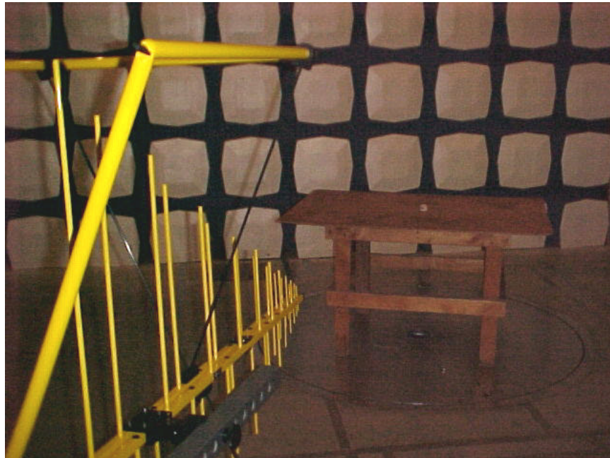
Figure 1. FCC Intentional Radiators Test Setup Photo
