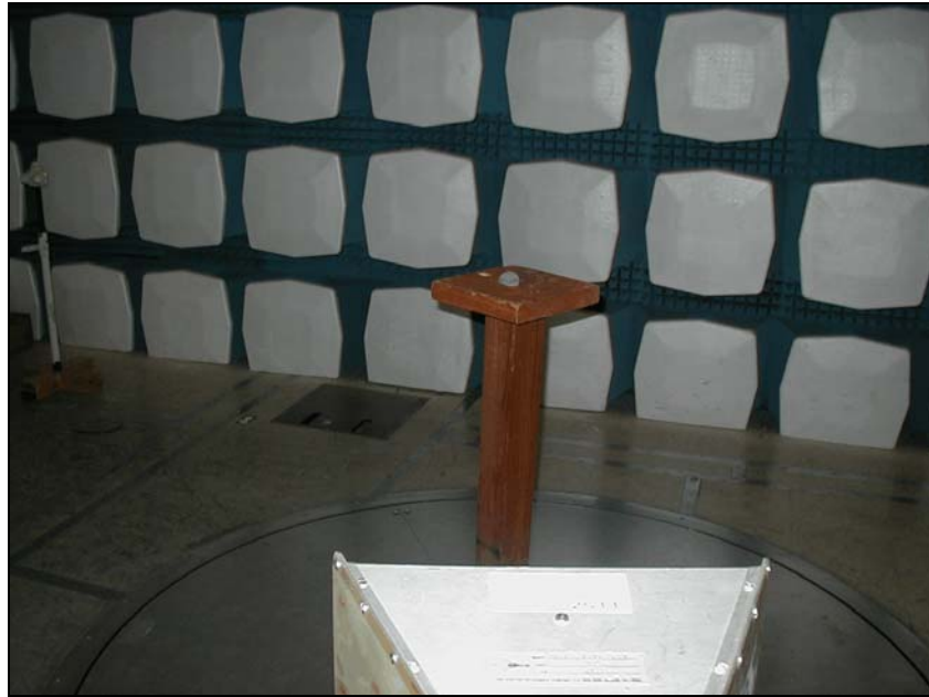
Photograph 3. FCC Intentional Radiators Test Setup Photograph 3
