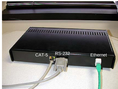
Figure 3. PAL-650 Hub and Power Distribution System.
