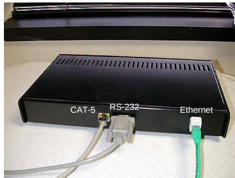
Figure 3. PAL-650 Hub and Power Distribution System.
