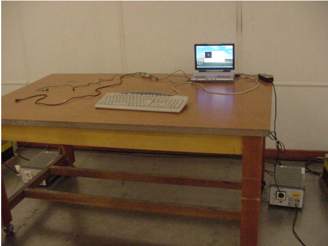
<FRONT PHOTO OF CONTINUOUS DISTURBANCE VOLTAGE >
