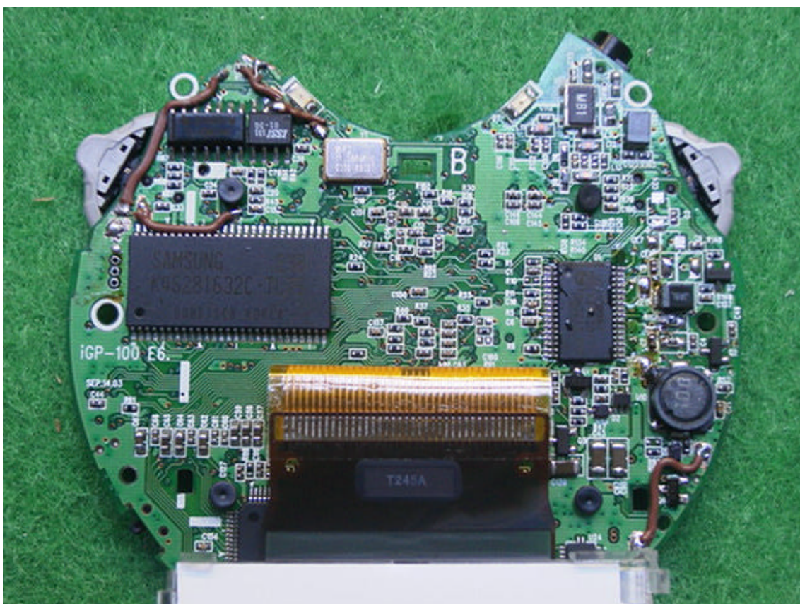
<FRONT SIDE OF MAIN BOARD>
