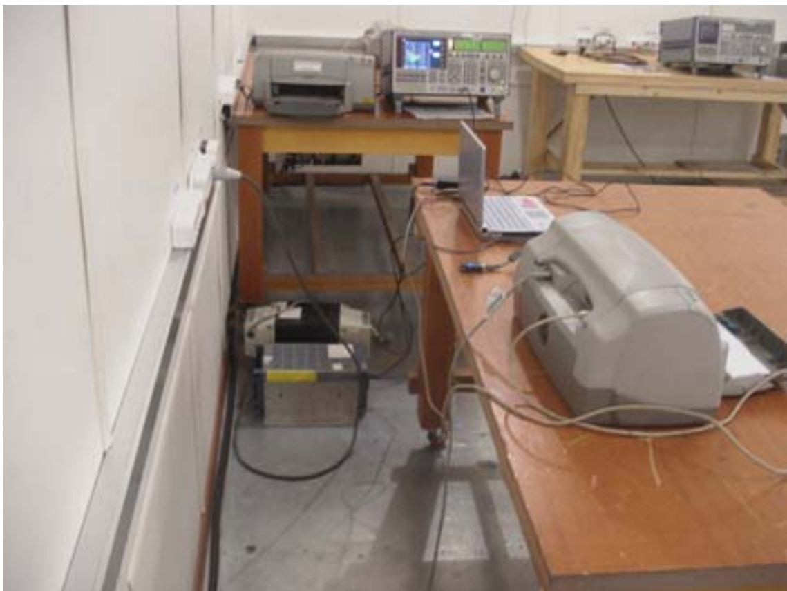
<SIDE PHOTO OF CONTINUOUS DISTURBANCE VOLTAGE >
