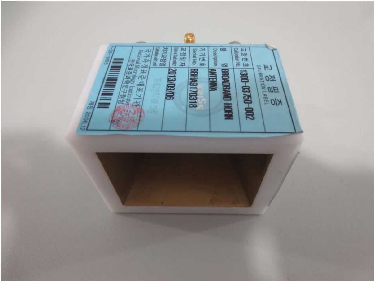
Horn Antenna(Antenna Spec: 15GHz~40GHz)
