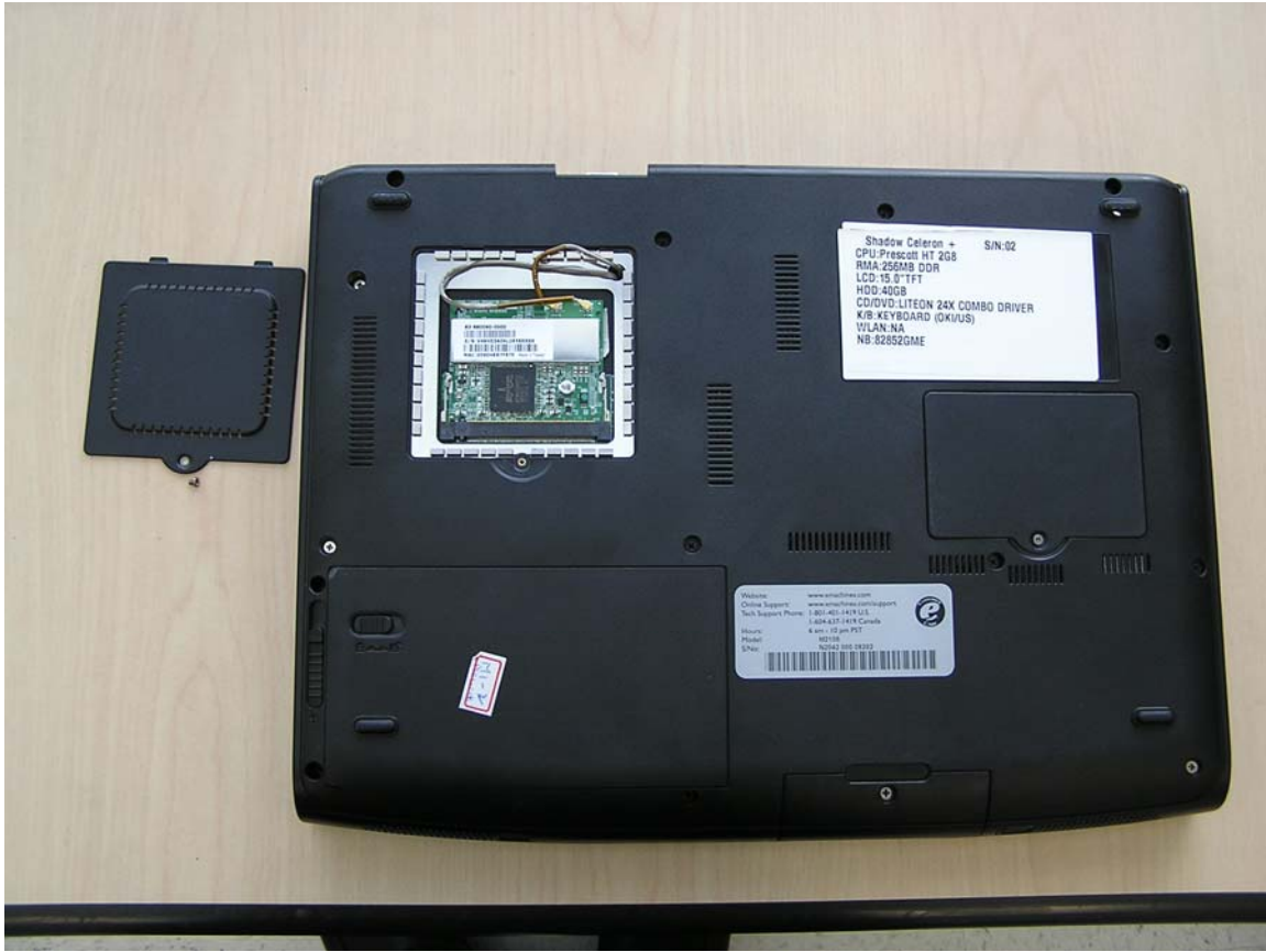
Laptop – bottom view showing location of WLAN
