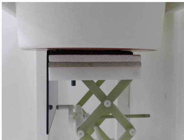
Bottom of Laptop, Test Separation 0 cm
