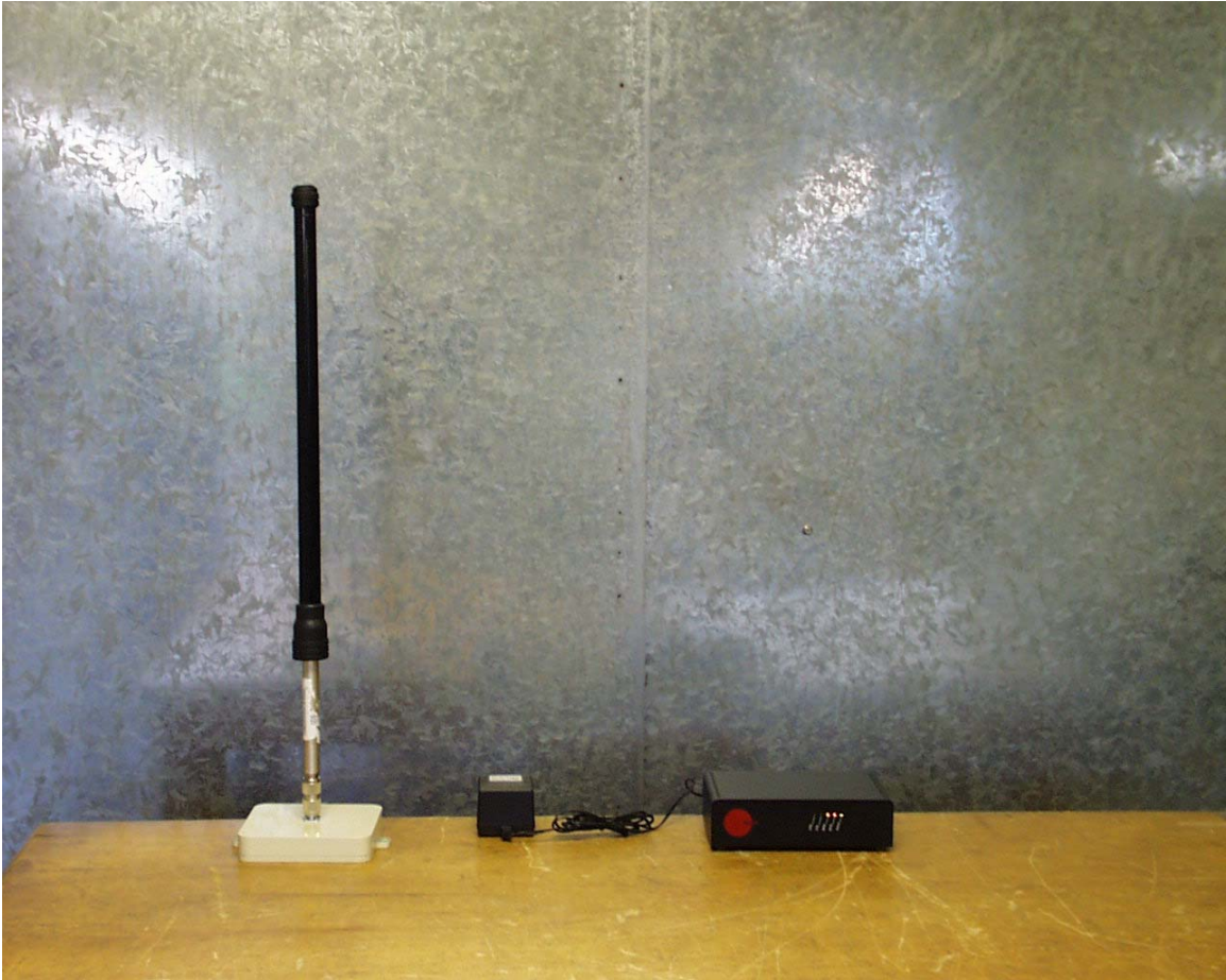
Line conducted test setup, front view
