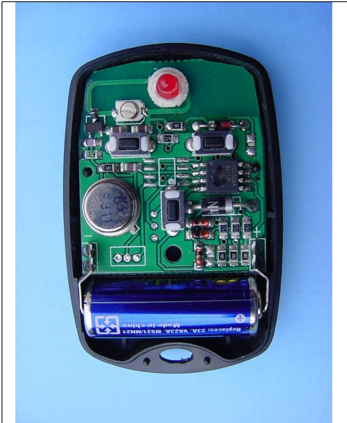
[ Inside View after Top Cover Open ]
