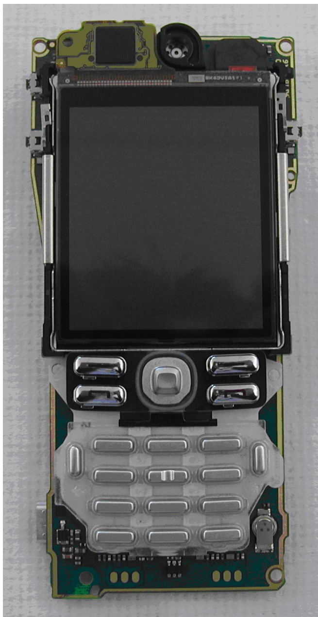
Fig 3 – PCB – Front View with Display and keymat
