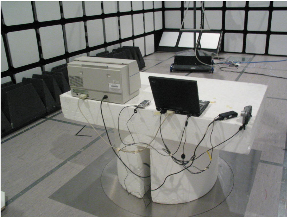
Picture 3 Radiated emission measurement (WLAN)
