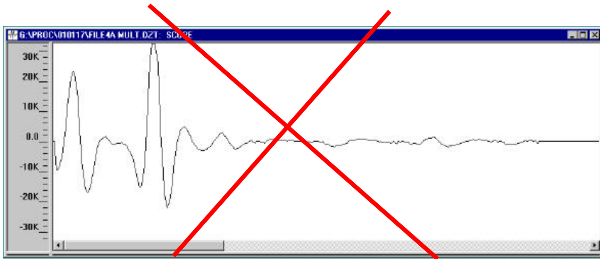
Figure 3: Example of Model 4108F data scan collected with too much gain.
