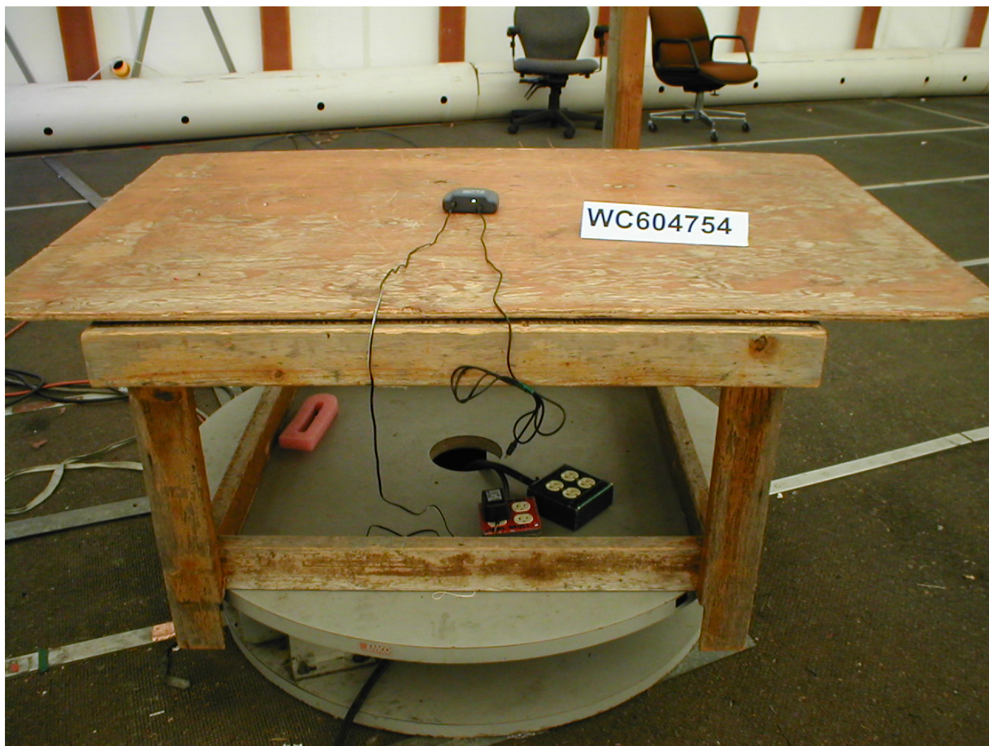
Test-setup photo: Radiated Emissions Model CLP-BMT1
