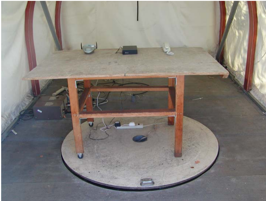
Base Radiated Emission - Front View
