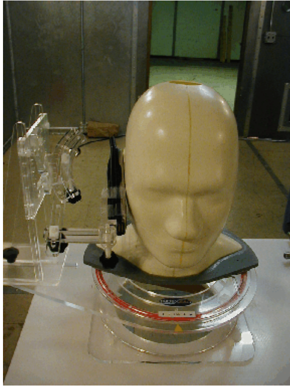
Figure S11. Configuration #11 - Cheek ( 0^{\circ} ) position, left side, GPS In, 1200 mAH Battery
