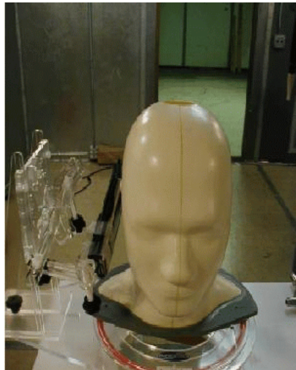
Figure S10. Configuration #10 - Tilt ( 15^{\circ} ) position, left side, GPS Out, 1200 mAH Battery
