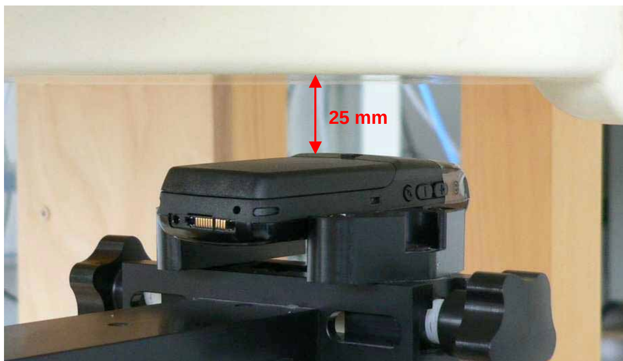
Fig. 22: Body worn configuration, GSM/ GPRS with and without BT activated, without accessory, antenna towards the phantom.
