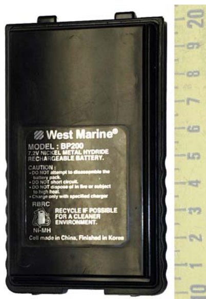
< Rechargeable Ni-MH battery pack, M/N:BP200, 7.2 V >
