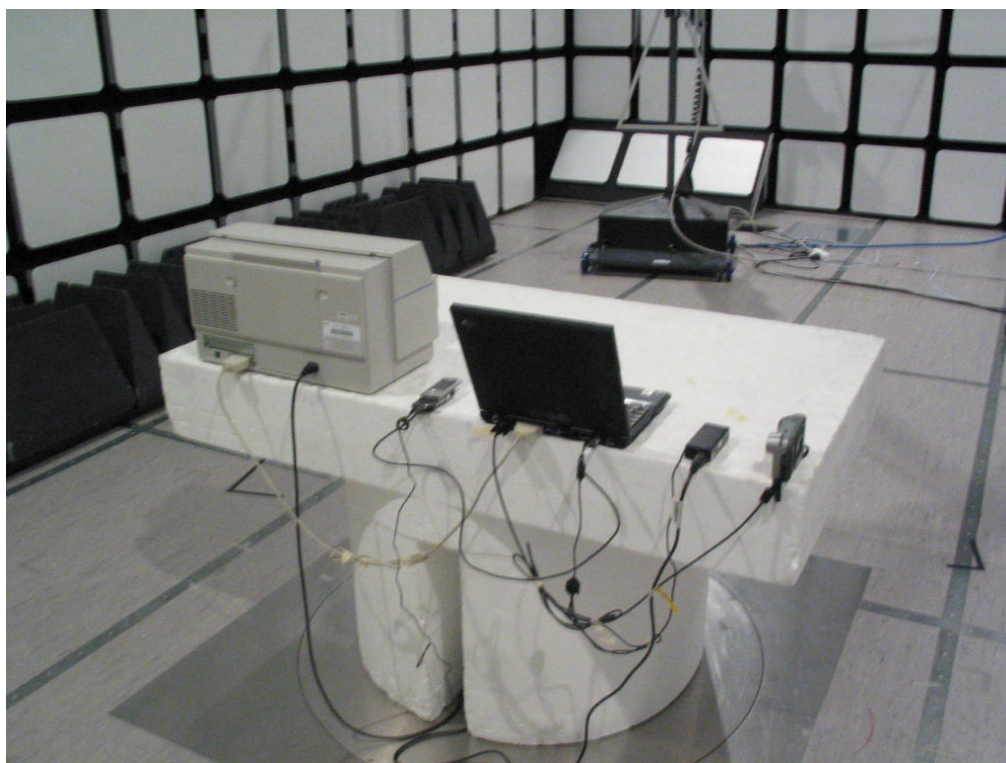
Picture 2 Radiated emission measurement
