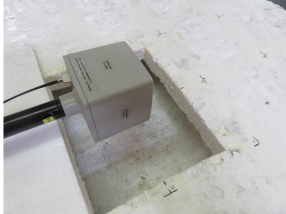
Photograph 8.1.2 Setup for RF exposure measurements, E-field
