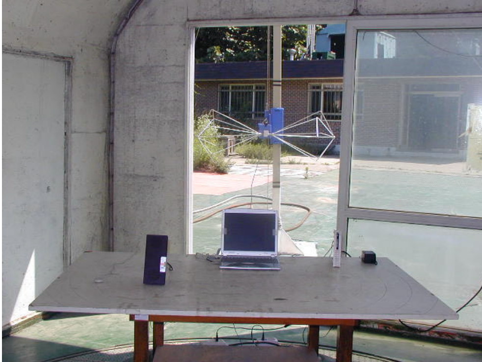
RADIATED EMISSION SETUP PHOTOGRAPH - FRONT VIEW ( 30 - 300 MHz )
