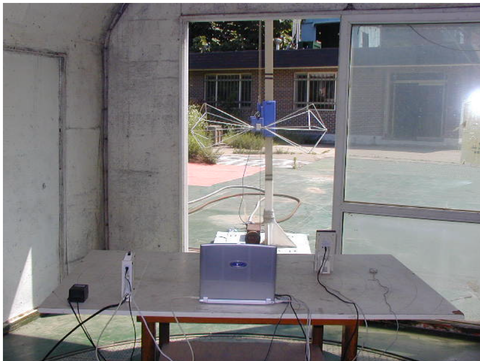
RADIATED EMISSION SETUP PHOTOGRAPH - REAR VIEW ( 30 - 300 MHz )
