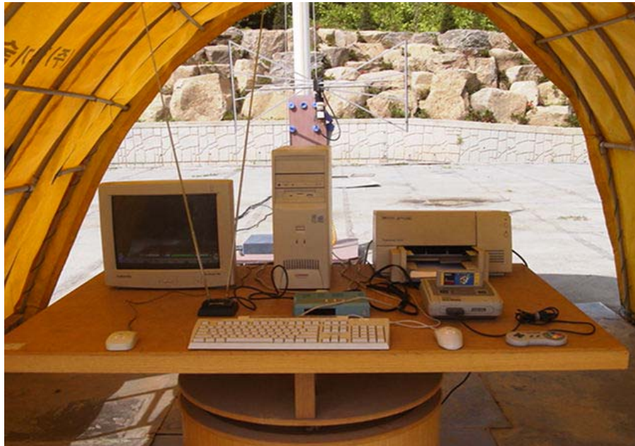
Photograph 1 : Setup for radiated Emissions
