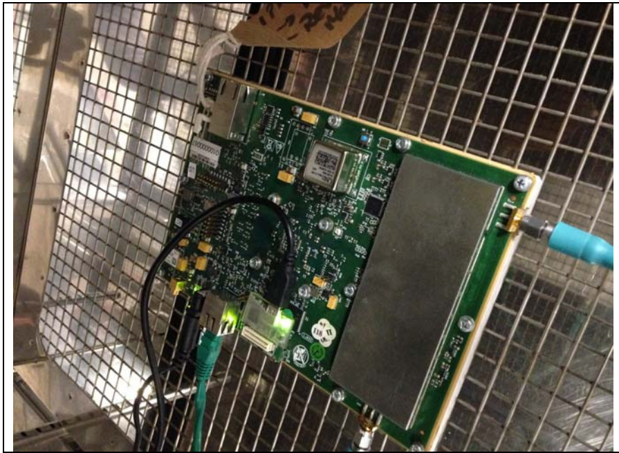
Fig 10 Test setup Temperature testing
