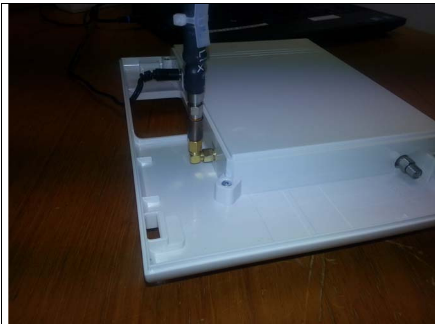
Fig 2 Test setup Conducted Emissions on Antenna port
