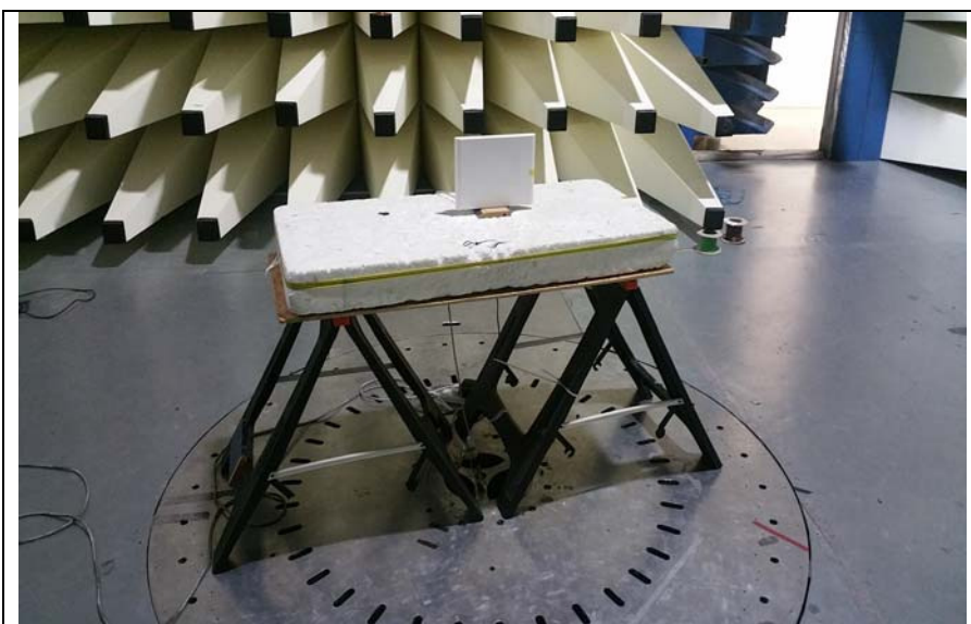
Fig 5 Test setup 30MHz -1GHz Rad Emissions
