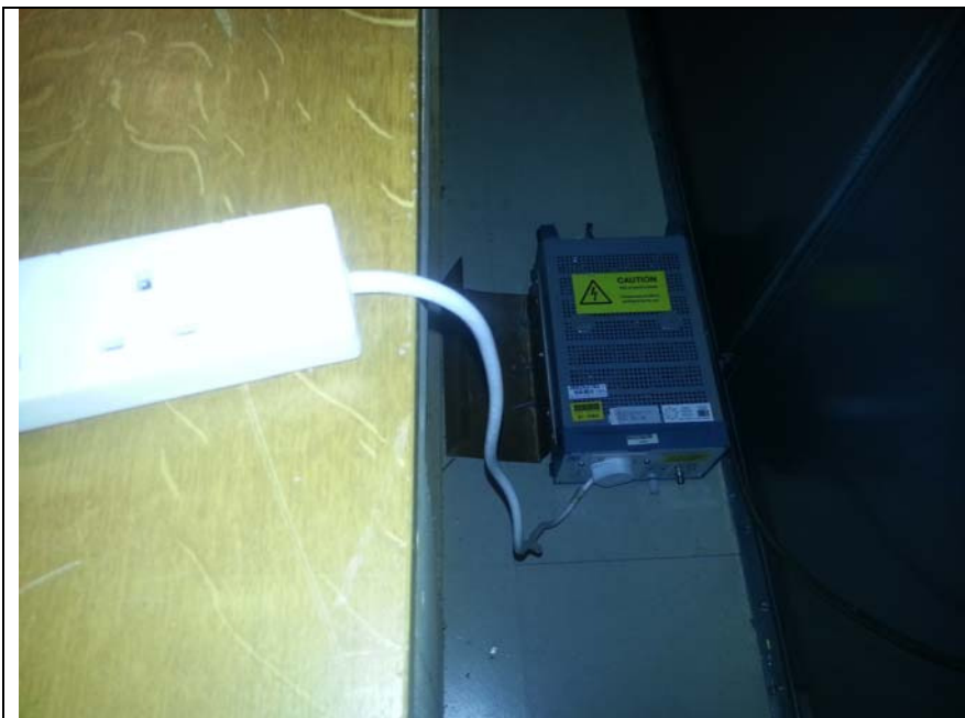
Fig 9 Test setup Conducted Emissions on the mains
