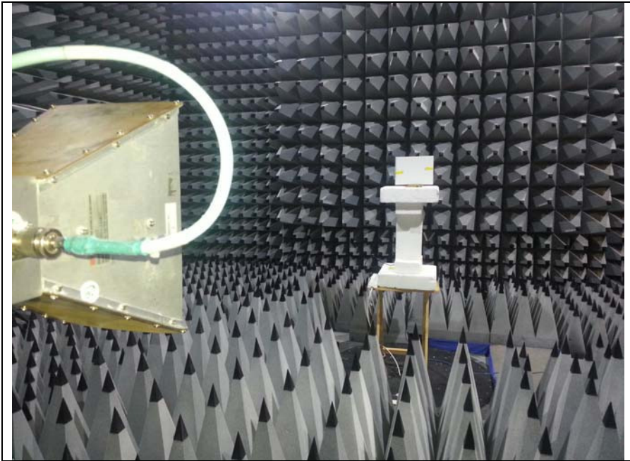
Fig 3 Test setup 1GHz -18GHz Rad Emission
