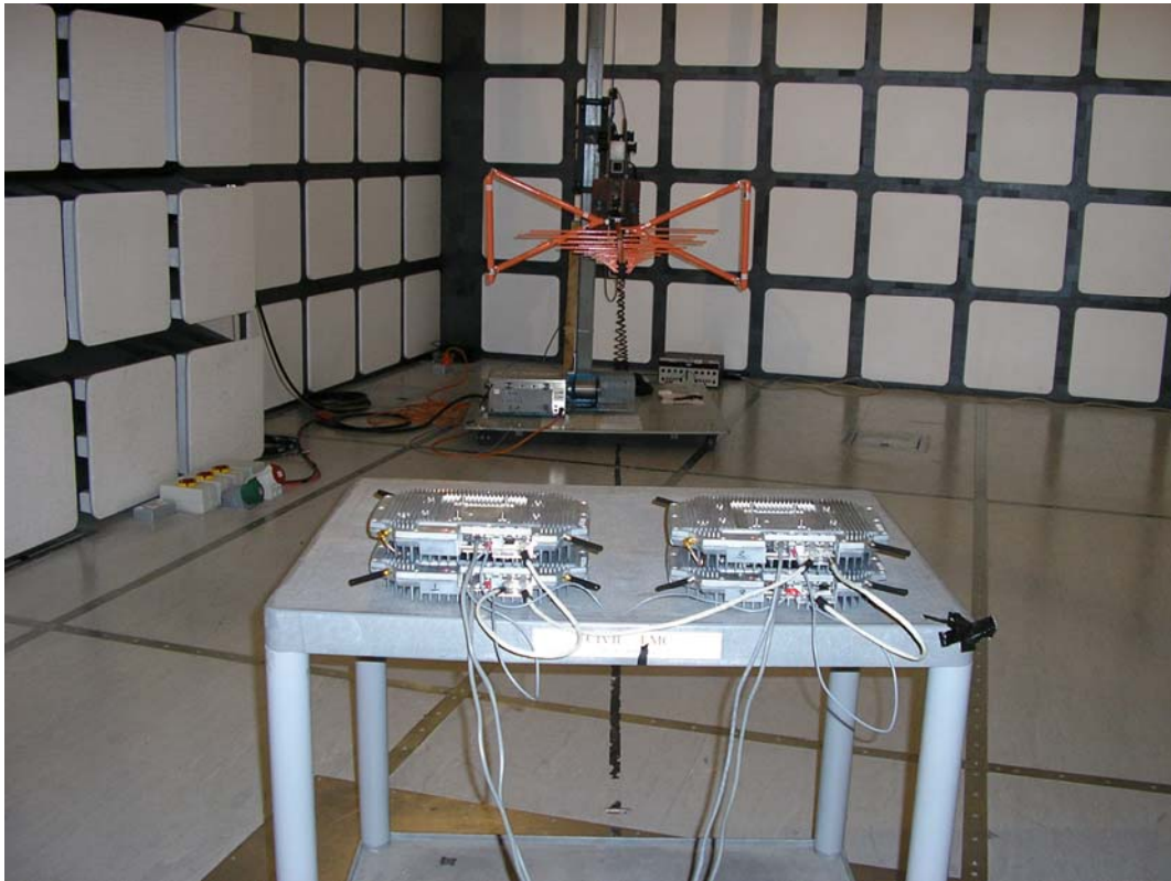
Radiated Emissions Test Set up
