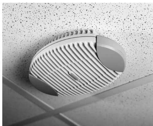
Figure 14 - Ceiling Mounted nanoBTS
