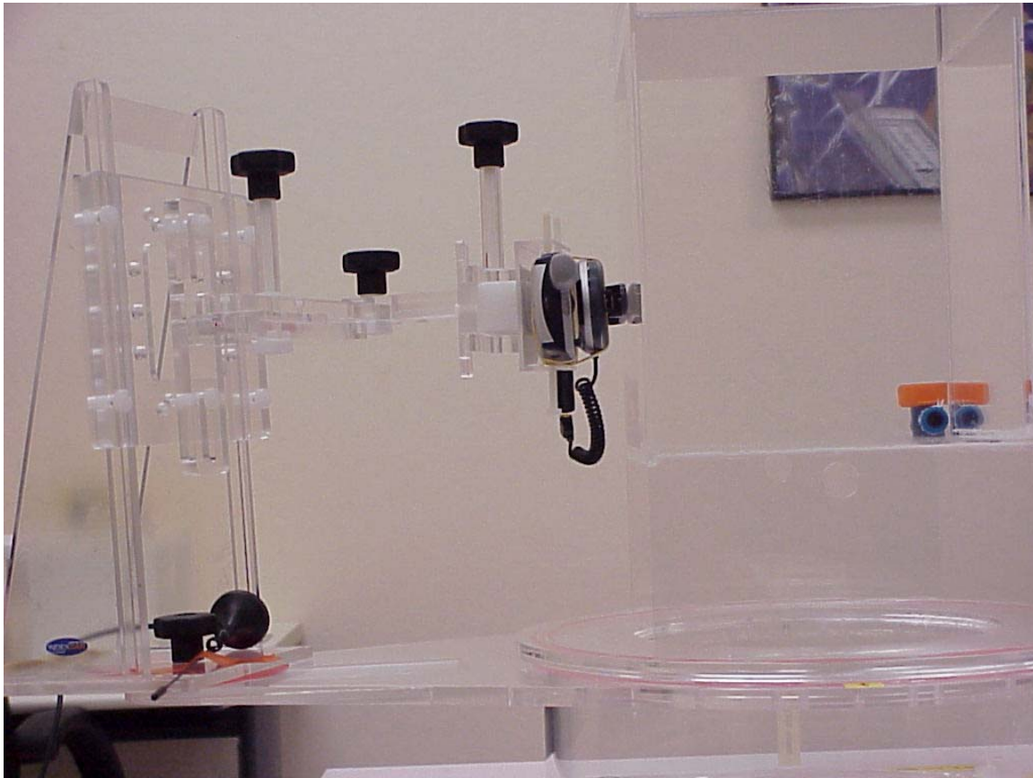
Photo 5: EUT belt clip configuration, EUT touching phantom.
