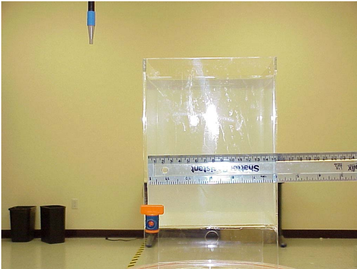
Photo 7: Photo to demonstrate 15 cm Z-axis flat phantom.
