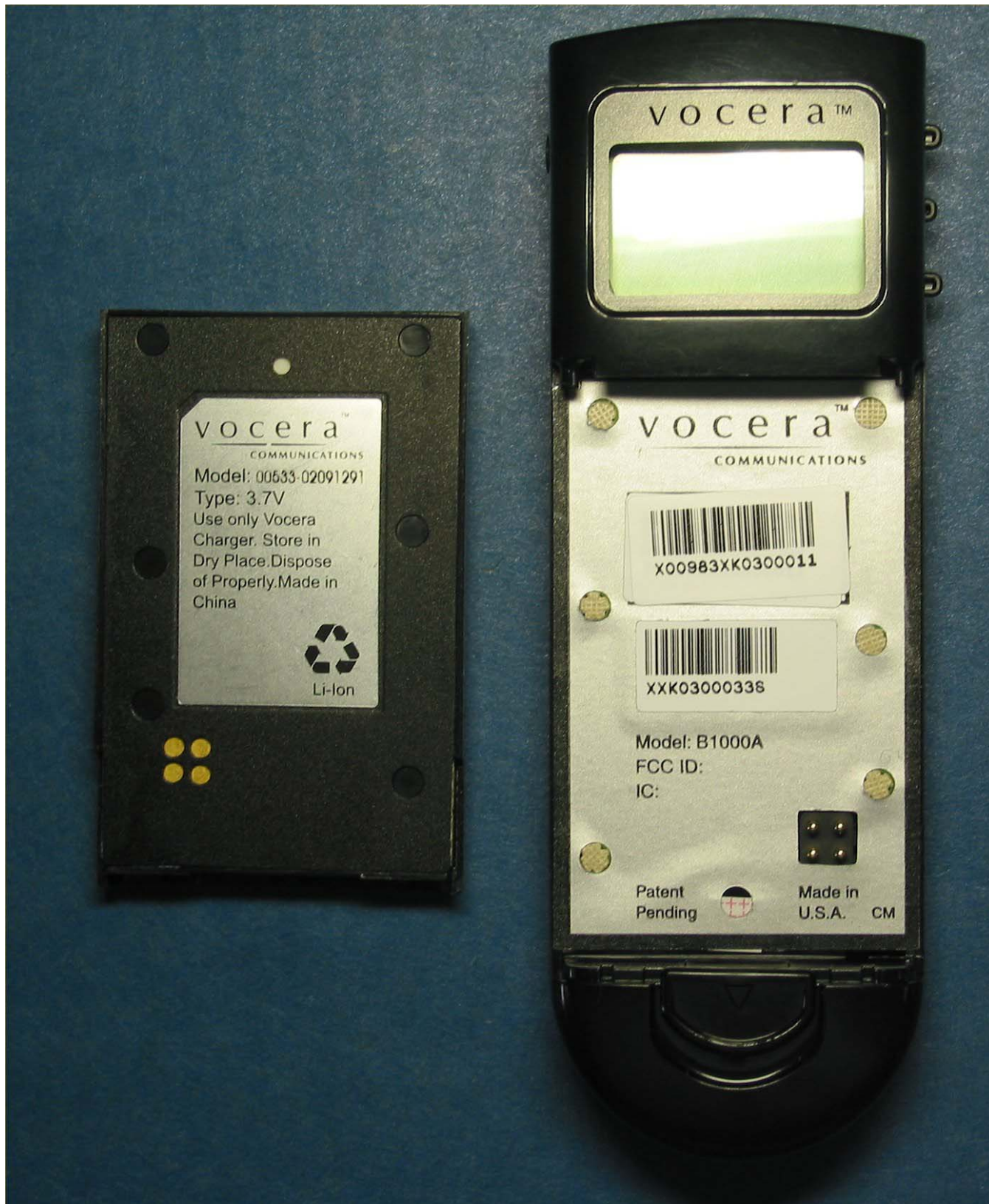
Vocera Communications badge, battery removed
