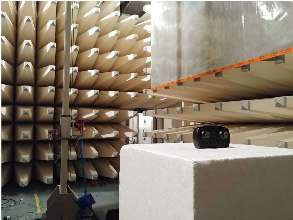
Set-up for Radiated Emission
