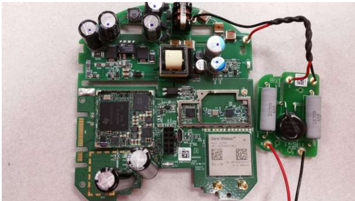
MODULE 574161 FRONT WITH SHIELDS REMOVED
