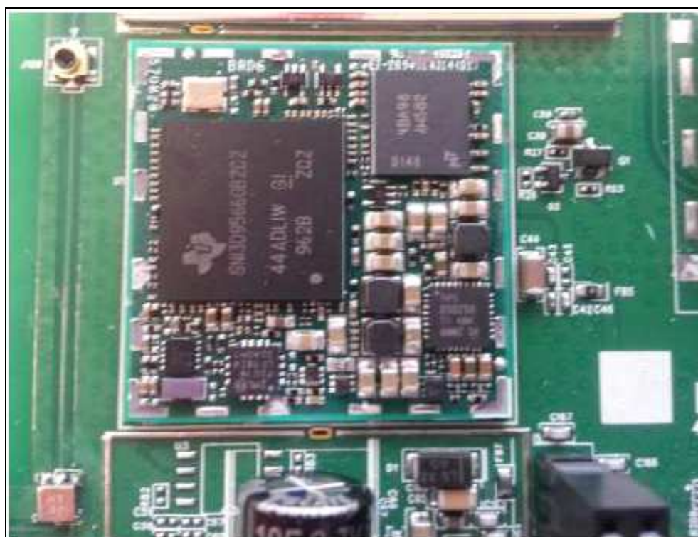
Figure 11: Internal Photo – ISOM Module U1 Shield Removed
