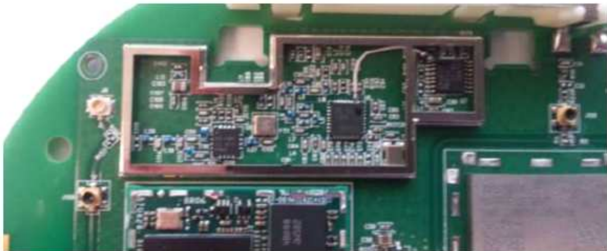
Figure 10: Internal Photo – 900MHz Radio Shield Removed
