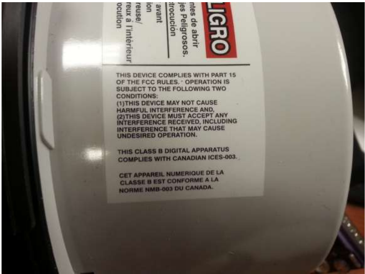
FCC & IC COMPLIANCE LABEL ON HOST METER
