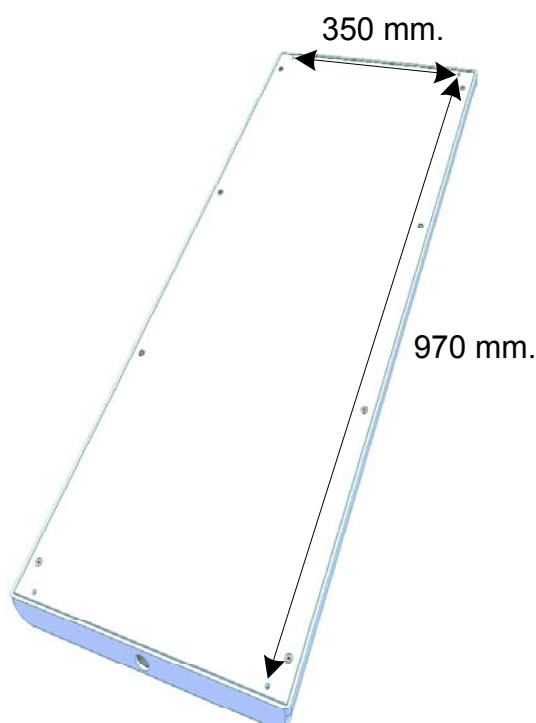
Figure 8: Conveyor Antenna Mechanical Diagram (Mounting Hole Dimensions)
