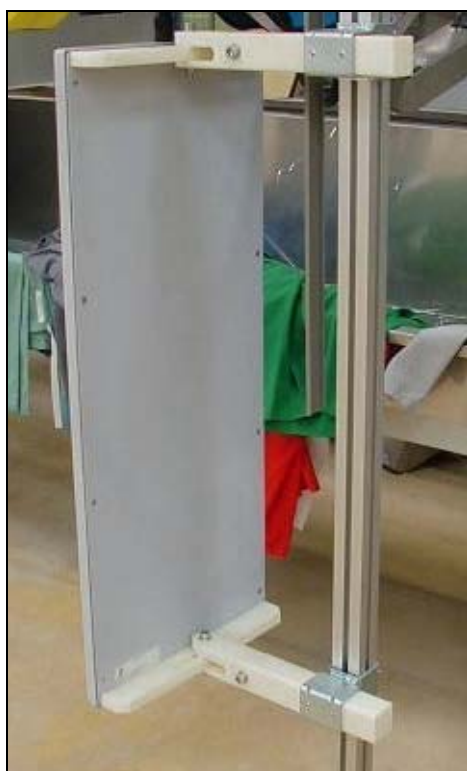
Figure 5: Mounting Brackets on Conveyor Antenna
