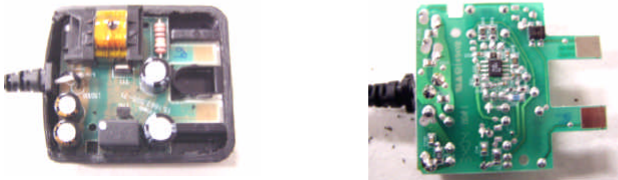
Power supply, cover removed
