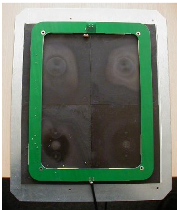
Figure 2: L-SA3 Antenna without Cover
