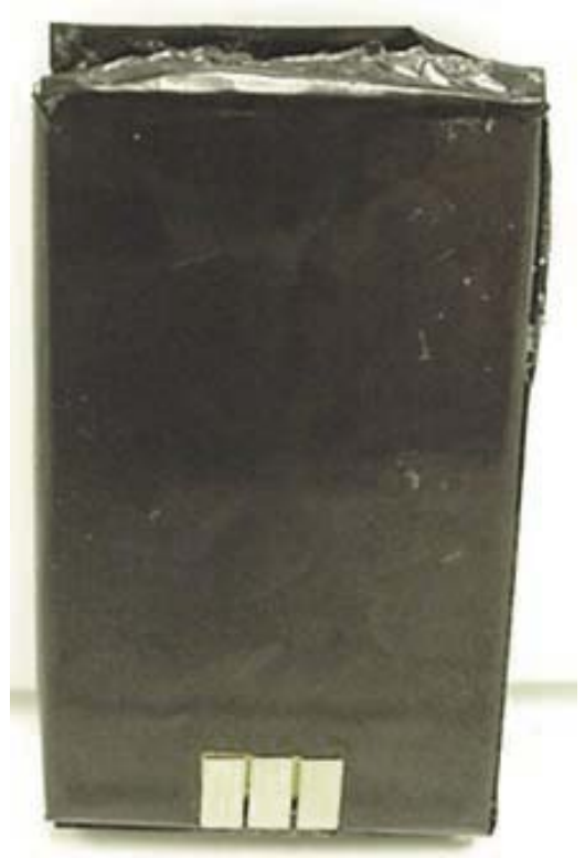
Lithium-ion Battery Pack
