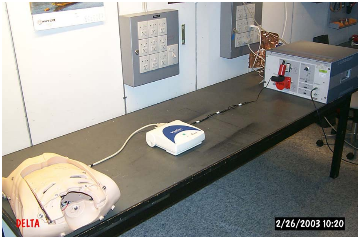
Photo 1 Set-up for measurements of conducted emission.
