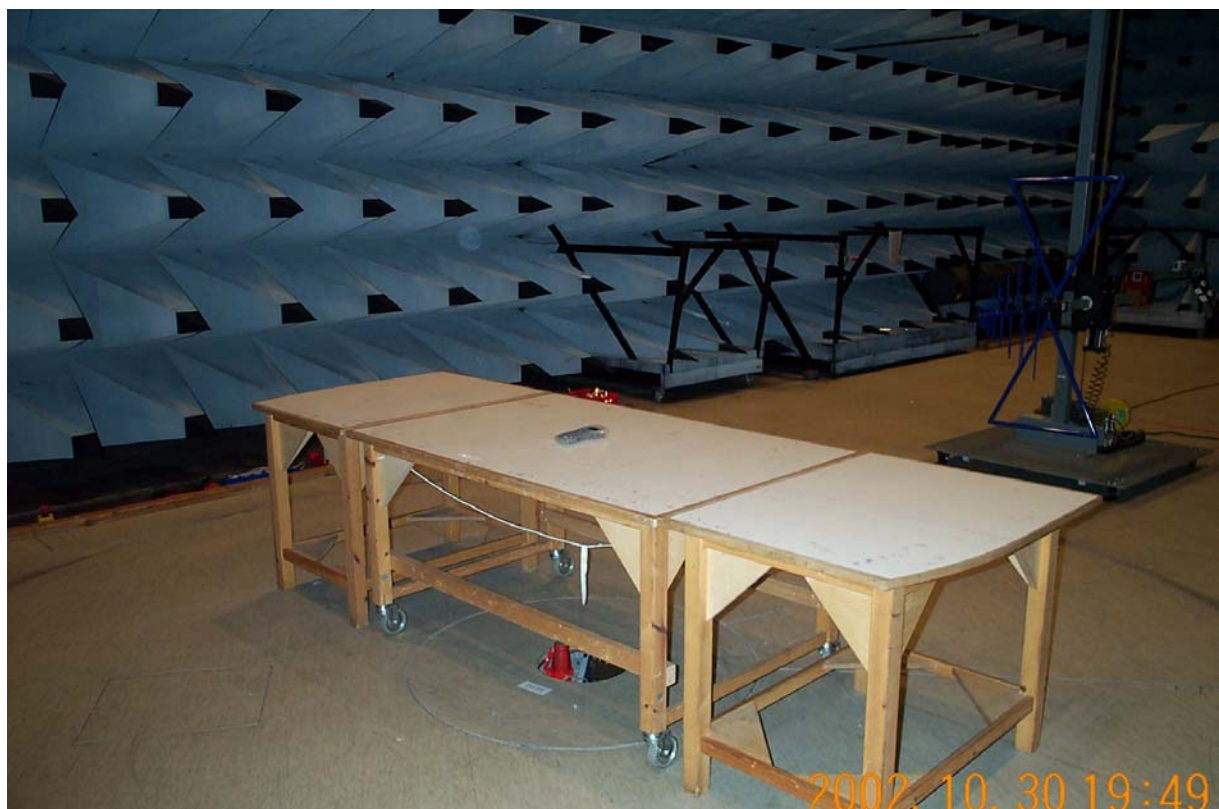
Photo 2 Set-up for measurements 30 - 1000 MHz.
