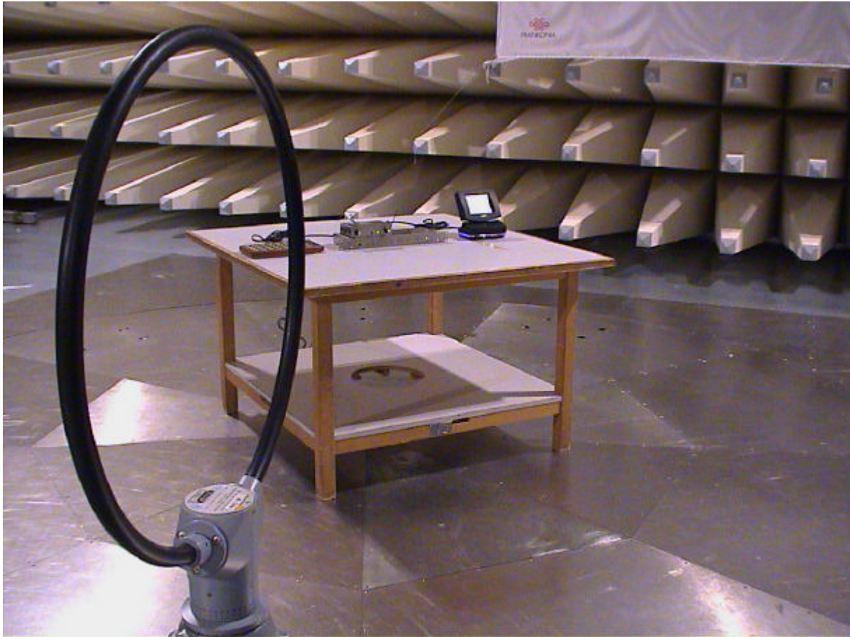
Fig. 1: Basic set-up for radiated emission; 9 kHz - 30 MHz
