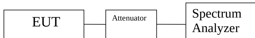
Figure 4. Block Diagram, Conducted Spurious Emissions Test Setup
