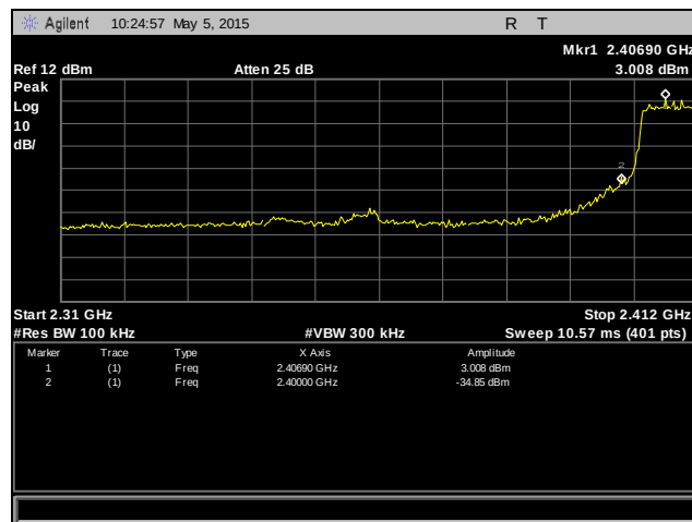
Plot 93. Conducted Band Edge, 802.11n 20 MHz, Low Channel, Port 1
