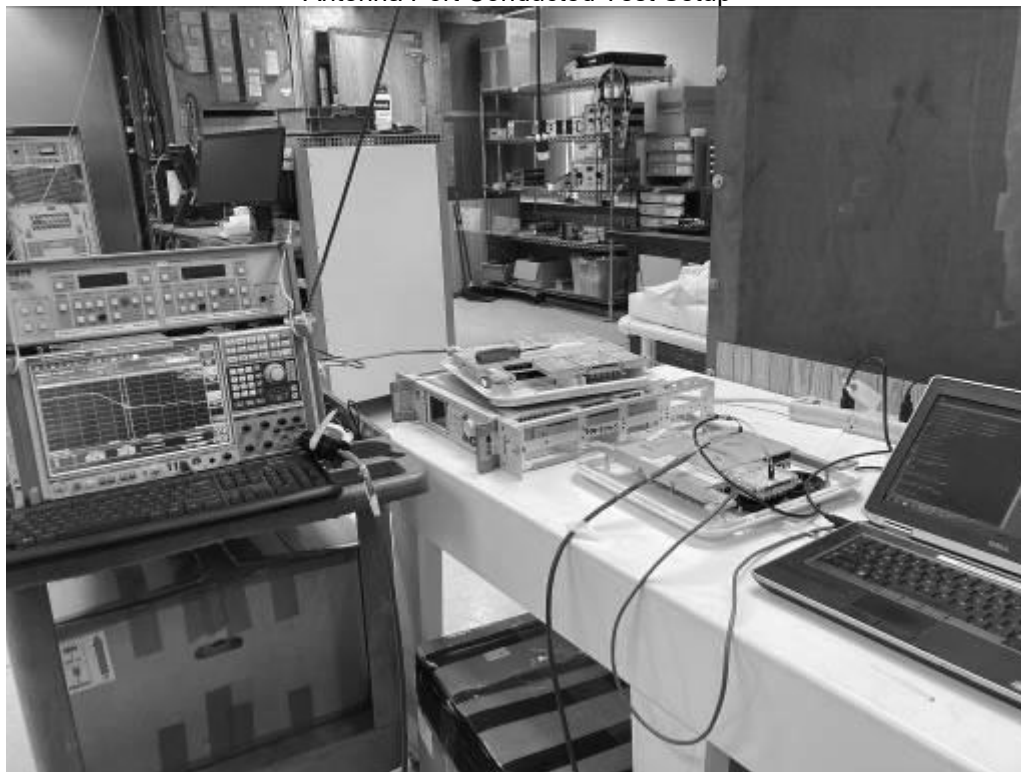
Antenna Port Conducted Test Setup
