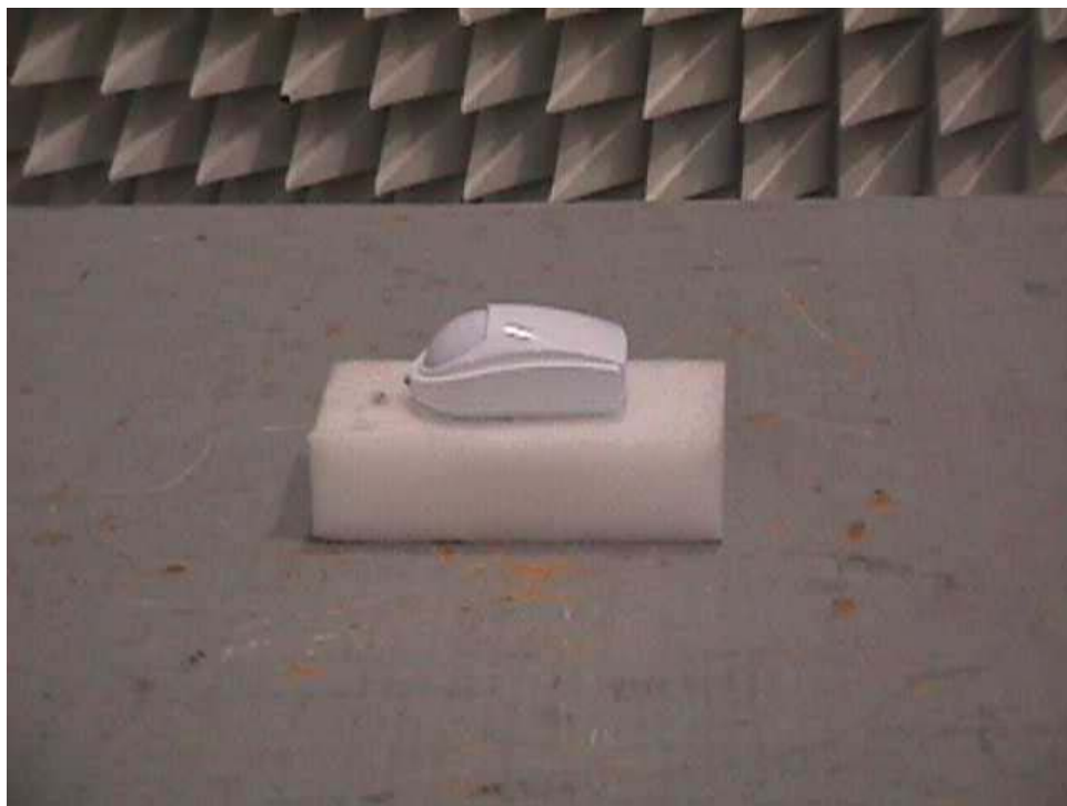
Radiated Emissions Test Configuration
