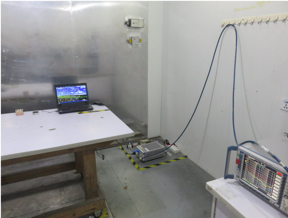
FCC RADIATED EMISSION TEST SETUP
