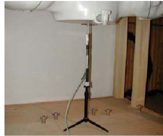
Figure 9.1 Dipole Verification Test Setup Diagram & Photo
