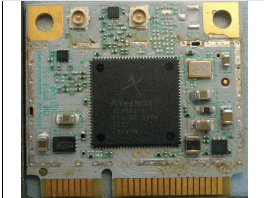
RF Module Top (removed shield)
