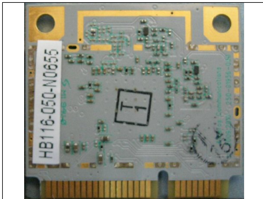
RF Module Bottom (removed shield)
