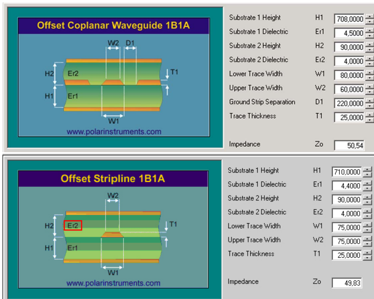
Figure 17: Embedded Stripline line arrangement
