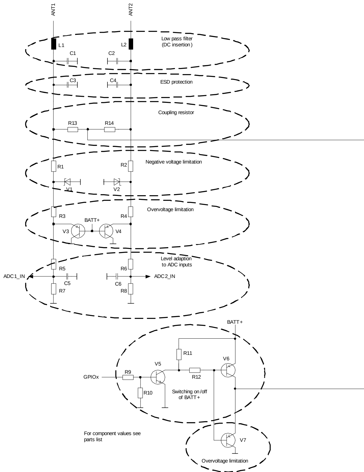
Figure 27: Antenna detection circuit sample - Schematic
